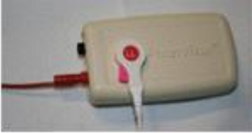
Photo 4: Pacerview device. Note EKG lead LL attached to Pacerview unit. G Dennis
